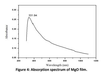
Fig 4 represents the UV-visible absorption spectrum of MgO film. This spectrum was recorded at the room temperature in the wavelength range from 200 to 1200 nm. To investigate the optical property of thin film is important for many industrial application. The absorption peak obtained at near ultra violet region in 331.9 nm which posses maximum absorption in lower wavelength. Due to wide band gap, maximum energy absorbed in lower wavelength region.
