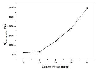
Figure 5: Sensing response variation of MgO film for different ammonia concentration
