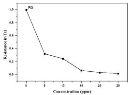
Figure 6:.Variation in electrical resistance of the film as a function of ammonia concentration.
