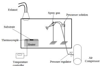
Figure 1: Schematic diagram of home built spray pyrolysis setup
