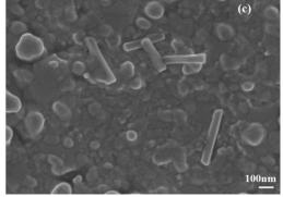
Figure 3: Field-emission scanning electron micrograph of MgO thin film at different magnification (a) 20,000 (b) 30,000(c) 40,000
